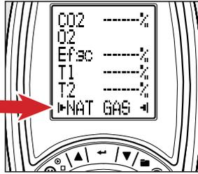
Press  $\blacktriangledown$  button until the Fuel Type displays on the Status Bar.
