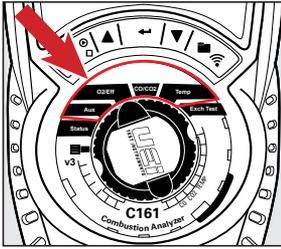
Rotate the dial to either AUX, O2/Eff, CO/CO2 or TEMP setting.
