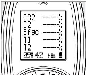
O2/Eff displays CO<sub>2</sub>, O<sub>2</sub>, Gross Efficiency, Flue temperature, Inlet temperature.
