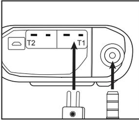
Insert flue probe into combustion input. Insert K-type temperature probe into input T1.
