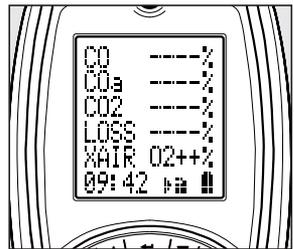
CO/CO<sub>2</sub> displays CO (ppm), Losses calculated, Excess air %. Make any adjustments needed for proper Combustion and wait for analyzer to display change in readings. (Repeat as necessary).
