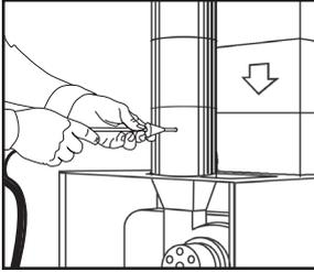
Remove the probe from the flue and allow analyzer to purge with fresh air until readings return to zero. O<sub>2</sub> to 20.9%, CO to Zero
