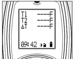
TEMP displays T1, T2 and Differential Temperature.
