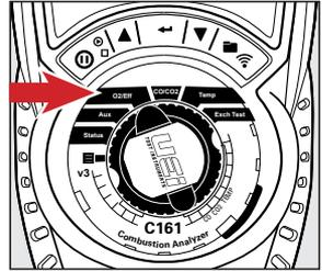
Rotate function rotary dial to O2/Eff for Test Screen 1 parameters.
